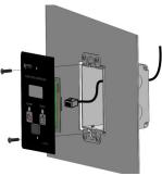
If the fume hood does not have a preinstalled electrical box available, then one will need to be installed.
